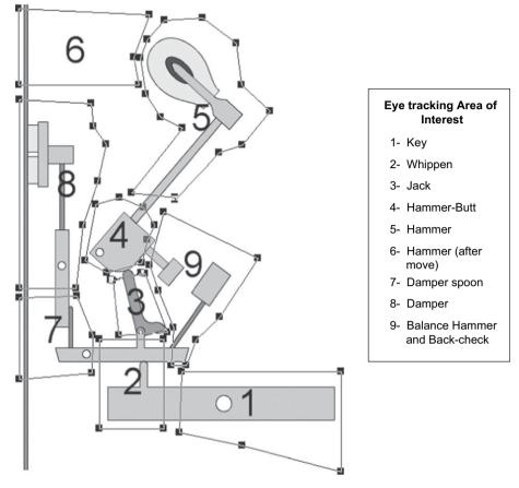
Fig. 3. The nine areas of interest for different piano mechanism parts.
