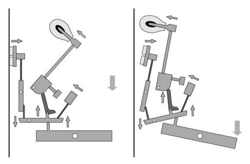
Fig. 1. Piano system with arrows indicating movement of parts.
