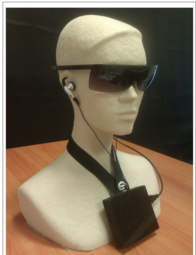
FIGURE 1 | Picture showing main parts of the sensory substitution device. An electronic eyeglass is connected to a battery-powered mini-computer that can be carried around the neck. This computer performs the signal transduction and generates sounds that are transmitted through running earphones.
